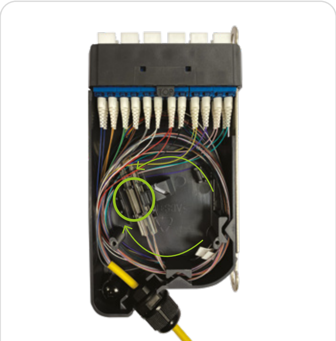
5 Proceed to splice. Once all fibers have been spliced, insert the gland into the cassette and secure. Secure the aramid tightly, making sure there is no slack with a strain tie to prevent movement and twisting of the pre-term. Note: We recommend coiling the fibers from the cable clockwise
