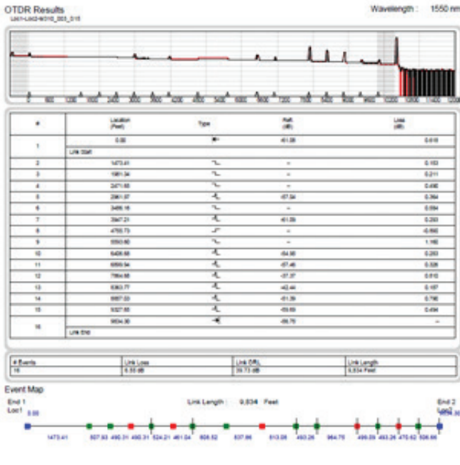
Figure 2—Event measurement results M310 vs. non-AFL OTDR for a 16-event network
