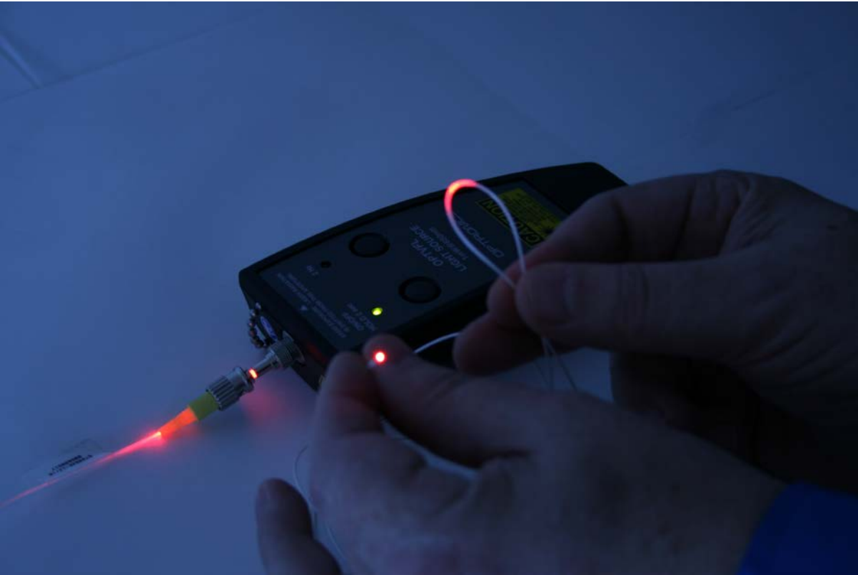
Picture 1: Detecting Macrobending with a VFL
